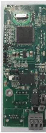
CANopen communication card EC-TX505/511
