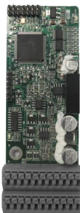
Resolver PG card EC-PG504-00
