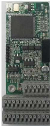
U/V/W incremental PG card EC-PG503-05
