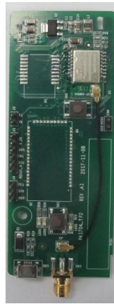
Bluetooth/WIFI communication card EC-TX501-1/50 2
