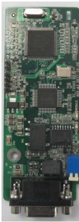
PROFIBUS-DP communication card EC-TX503
