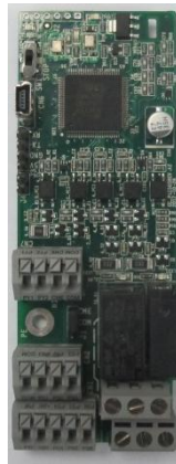
Programmable extension card EC-PC501-00
