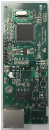
Ethernet communication card EC-TX504
