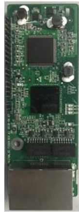
PROFINET communication card EC-TX509
