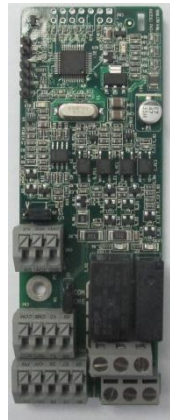
IO extension card EC-IO501-00
